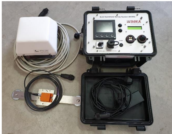
MOSS unit (right-top) with motion sensor (left-bottom) and IRIIDIUM unit (left-top)
