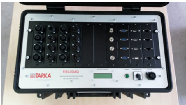
FIELDDAQ front with multiple individual connector plates
